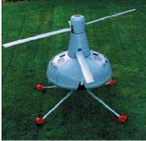
Fig. 3. Remotely piloted vehicle (developed at EA Technology Ltd).
