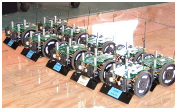
Fig. 1. Ten Mica2-based robots for the MAS-net project.
