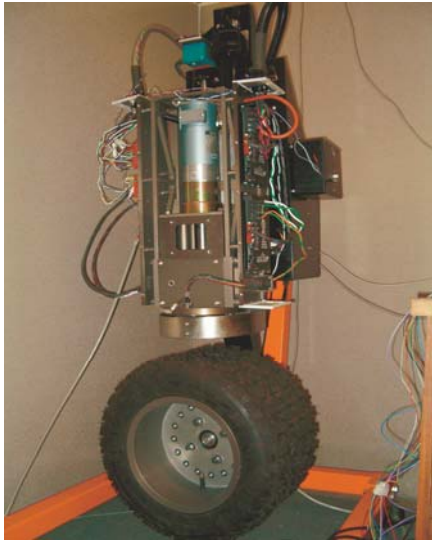
Fig. 1. Smart Wheel Assembly on a Mobile Rig.
