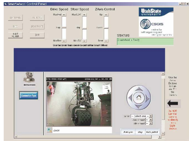
Fig. 3. Screen-shot of the Telepresence Control System Application.
